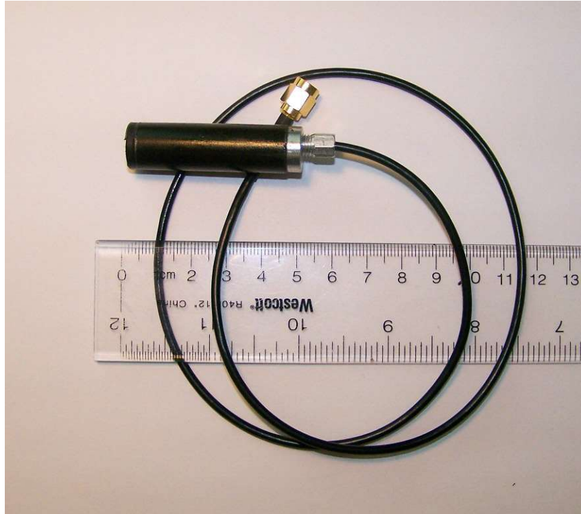
Fig. 6. Miniature focusing transducer for operation in pulse – echo mode. The transducer contains installed cable RG-174/U (length ~ 60 cm) with SMA connector at the end. There may be applied other connector – BNC. Diameter of the housing is 13.2 mm.
