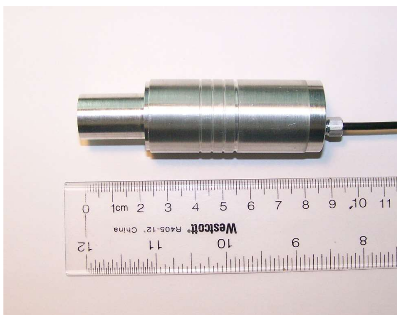
Fig. 4. Power ultrasonic transducer with work frequency 100 kHz. Diameter of the taper is 6 mm, diameter of the housing is 25.4 mm. Diameter of the taper can be done larger – up to 12 mm.
