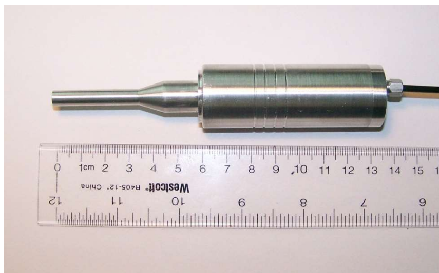
Fig. 4. Power ultrasonic transducer with work frequency 100 kHz. Diameter of the taper is 6 mm, diameter of the housing is 25.4 mm. Diameter of the taper can be done larger – up to 12 mm.
