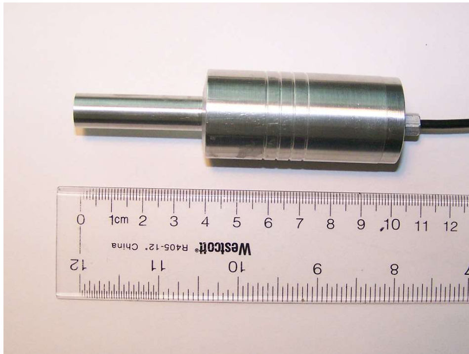
Fig. 3. Tapered power transducer with diameter of the taper 10 mm. Diameter of the housing is 25.4 mm. Each transducer has water protected Aluminum housing with installed coaxial cable RG-174/U (~1.2 m) and BNC connector at the ends. Connection of such coaxial connector with the cable is shown on Fig. 2 in section “HIFU transducers in closed metal housing”.
